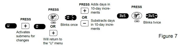
A. Press the Menu button three times to display the CLEARRAY Bulb Replacement Timer Menu. The LED screen will display "U."
